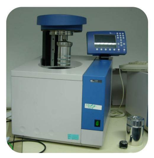
Though not particularly beautiful machines, calorimeters are incredibly useful ones. They are used to determine the calories (food energy) in food, as well as the average heat yield from burning various grades of coal and oil. The price of coal is often dependent on the heat yield from samples burned in a calorimeter.
