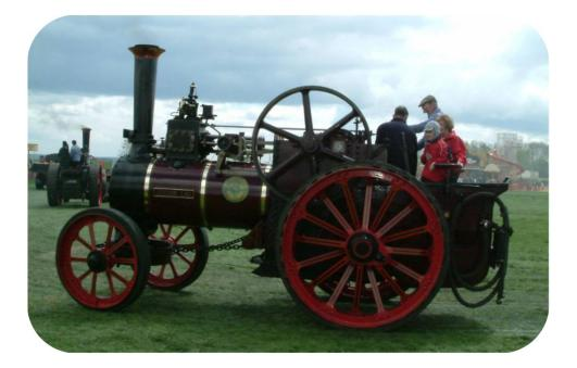
Before the internal combustion engine was invented, steam engines were the power source for ships, locomotives, tractors, lumber saws, and most industrial machines. Coal or wood was burned to boil water into steam, which ran the engine.
