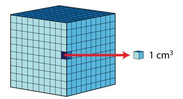
As seen in the illustration above, the volume of 1,000 blocks, each with a volume of 1 cubic centimeter, is equivalent to 1 liter.
