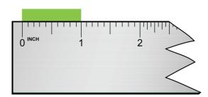
In this second case (sketch above), it is apparent that the object is, as nearly as we can read, 1 inch. Since we know the tenths place is zero and can estimate the hundredths place to be zero, the measurement should be reported as 1.00 inch. It is vital that you include the zeros in your reported measurement because these are measured places and are significant figures.
